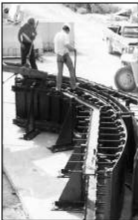
Modular formwork for precast arches produces a wide variety of shapes and sizes
